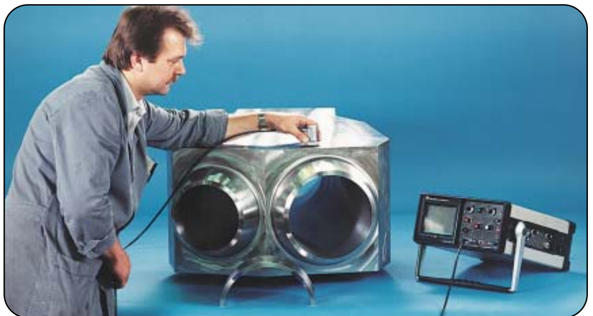
Wye Piece in Böhler A911 for offshore application
