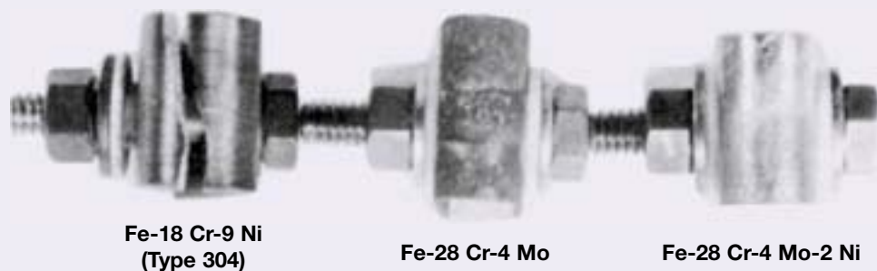
Figure 43 Welded U-bend specimens exposed for 134 hours in 50% NaOH solution at 200°C 28
